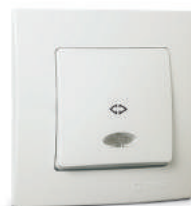
Intermediate Switch Illuminated * 32001040 10 AX, 250 V~ EN 60669-1 Piece in Box / Package - 12 / 120
