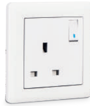
Socket-Outlet Switched 2P Illuminated BR022001 13 A, 250 V~ BS 1363-2 Piece in Box / Package - 12 / 120
