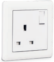
Socket-Outlet Switched 2P BR021901 13 A, 250 V~ BS 1363-2 Piece in Box / Package - 12 / 120
