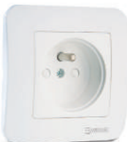
Socket Outlet with Earthing Pin and Child Protection * 55053 16 A, 250 V~ IEC 60884-1 Piece in Box / Package - 12 / 120
